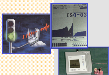
Fig 1 : Principle of the Osstell. An ISQ value is obtained, it should orient the practitioner versus IL or versus DL (Fig 1).
